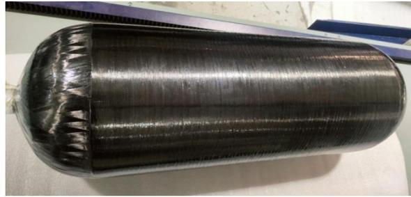
Figure 6: Fabricated Type 3 composite Cylinder prototype by Indian Oil
