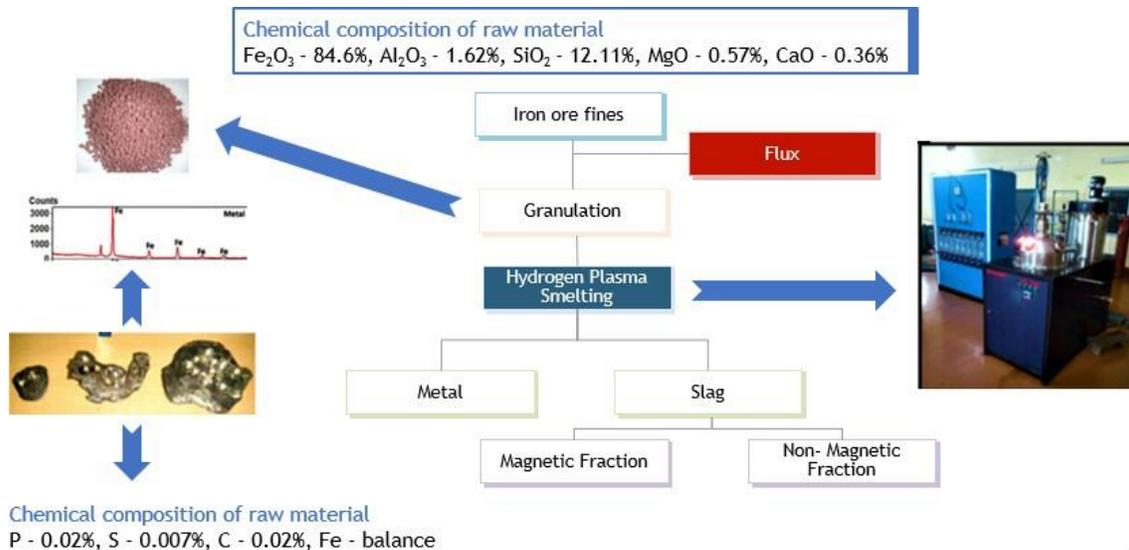
Figure 15: Process flow chart for green steel production
