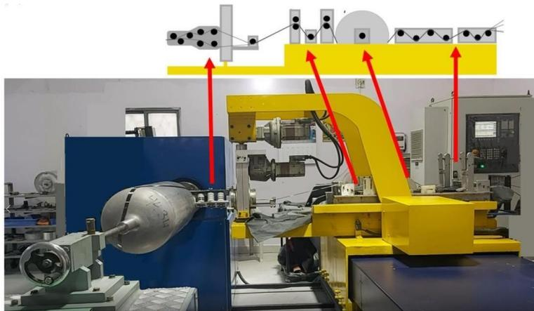
Figure 4: Filament winding machine
