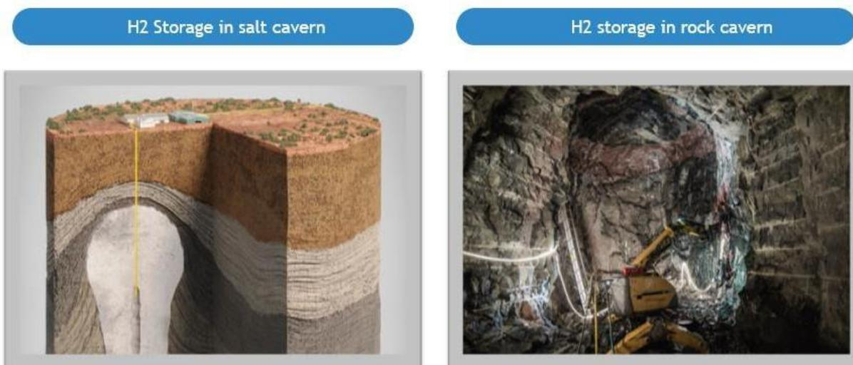
Figure 3:a). H<sub>2</sub> Storage in a salt cavern, b). H<sub>2</sub> storage in rock cavern (Source: Google)
