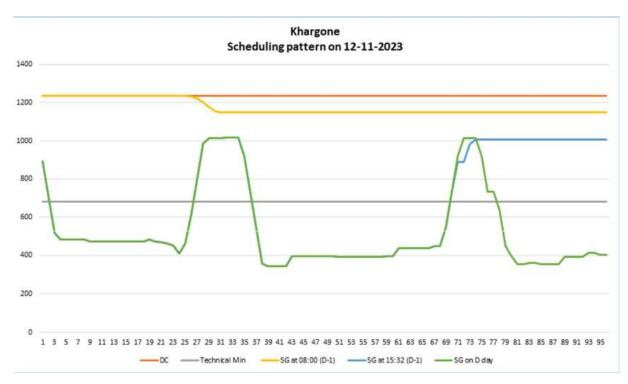
Due to the full schedule on 'D-1' day, the generator is not able to bid the URS in DAM, restricting the participation of the unit in SCUC provisions/MOD stacking of stations and also USD planning on D-1 day. Therefore, the downward revision of the schedule by the buyers be limited up to the Minimum turn down level.
